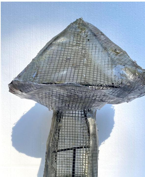
3. Fiberglass and resin hardened over the form
